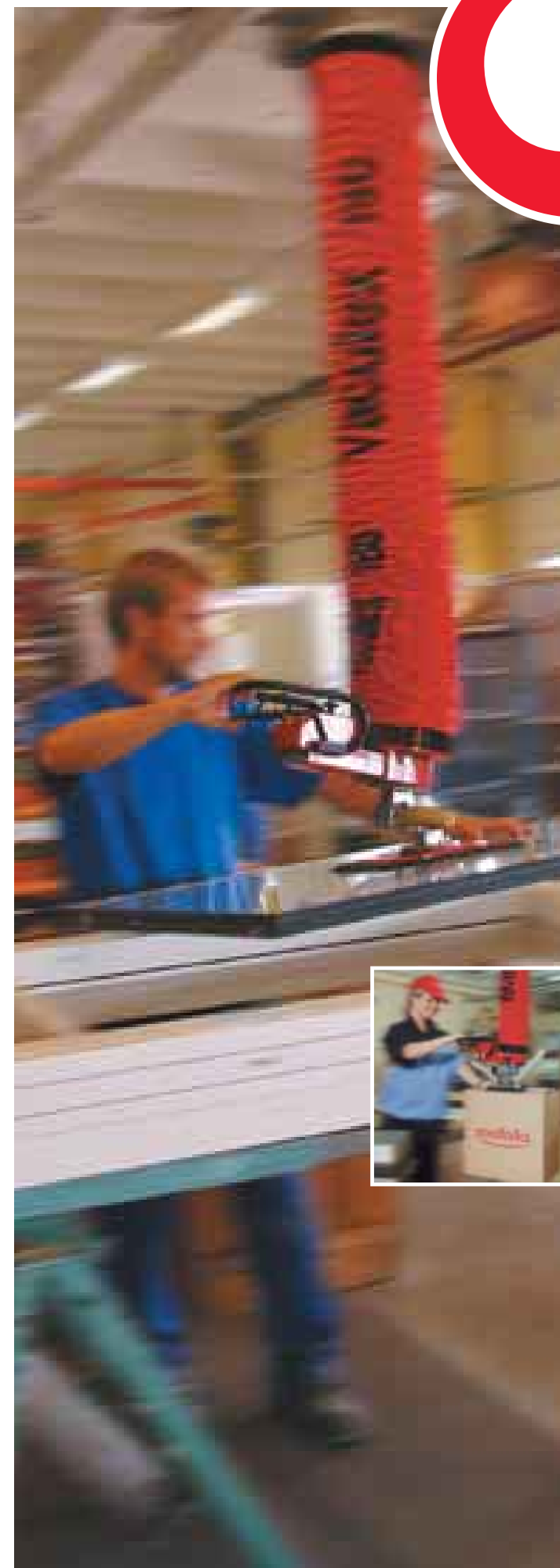
The vacuum tube lifters are easy to install and can be adapted to lift virtually any object – for instance boxes, sacks, panes of glass, sheet metal, stone slabs, drums, barrels, cans, computers etc.
